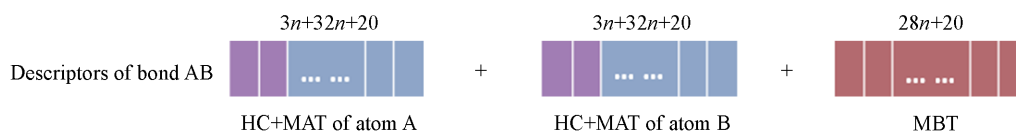
Fig. 6 Composition diagram of the HAB descriptor
