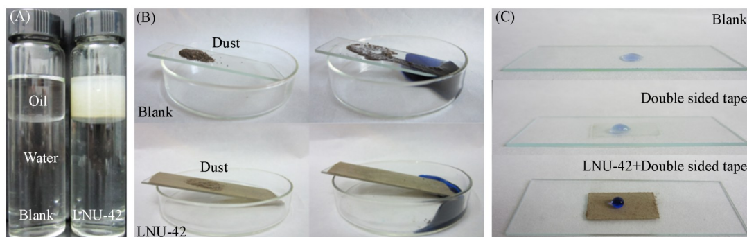
Fig. 3 Photograph of LNU-42 solids dispersed in a kerosene/water mixture(A), self-cleaning performance of LNU-42(B) and water(dyed with methylene blue) droplets on the LNU-42 coated glass(C)
