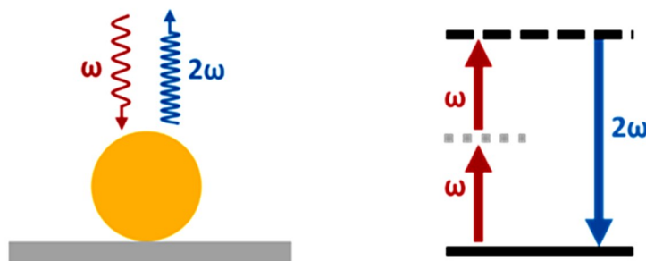
Fig. 1 Schematics of second harmonic generation, as the representative example of the non-linear optical processes
