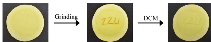
Fig. 5 Schematic representation of information storage and erasure in [\text{AuCu}(\text{L})_2]_n -based paper
