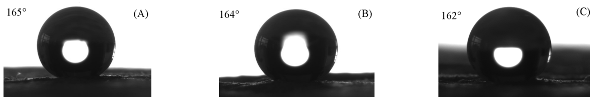
Fig. 3 Photographs showing the water contact angle of the paper modified by perfluorooctyl azide copolymer-80 in 0 h(A), 24 h(B) and 48 h(C)
