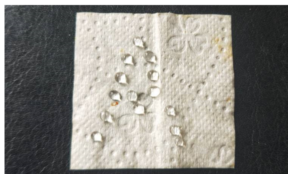
Fig. 5 Superhydrophobic effect of the paper modified by perfluorooctyl azide copolymer-80
