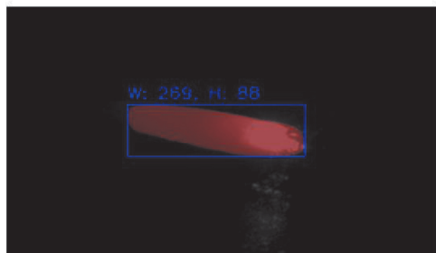
(c) 基于Deeplab v3+的熔池轮廓尺寸提取
