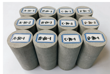
图 4 青砂岩试件(冲击加载试验) Fig.4 Green sandstone specimens (impact loading test)
