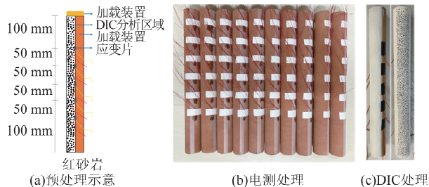
图 7 红砂岩试件及电测、DIC 预处理示意 Fig. 7 Red sandstone specimens and DIC pretreatment diagram
