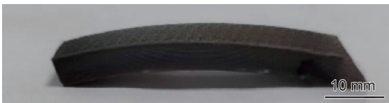
图 16 填充率60% 烧结样品形貌 Fig.16 Morphology of sintered samples with a filling rate of 60%
