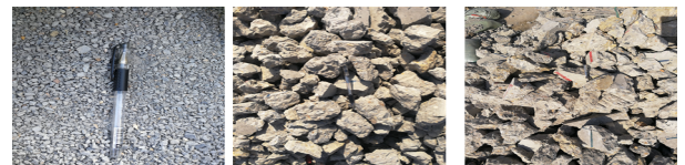
(a) d < 5 \text{ mm} (b) 5 \text{ mm} \leq d \leq 100 \text{ mm} (c) d > 100 \text{ mm}
