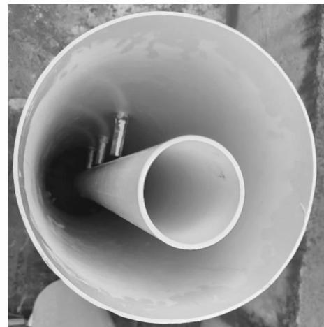
图 14 厚壁圆筒应变片布置图 Fig. 14 Strain gauge layout on the thick wall cylinder
