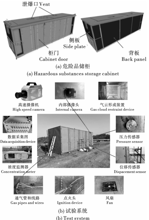
图 2 危险品储柜及甲烷爆炸试验系统 Fig. 2 Hazardous substances storage cabinet and methane explosion test system
