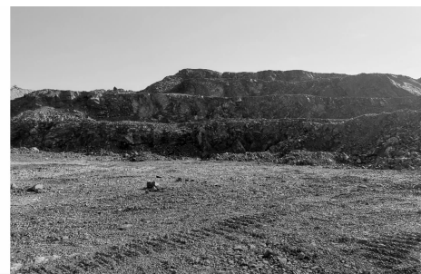
图5 爆破新台阶面 Fig. 5 Bench surface after bursting blasting
