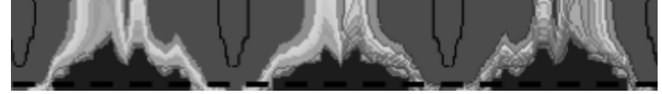
图3 超深0.4 m条件下爆后新台阶面的起伏分布图像 Fig. 3 The undulation distribution image of the new step bench surface after explosion blast under the condition of subdrilling ultra-deep 0.4 m
