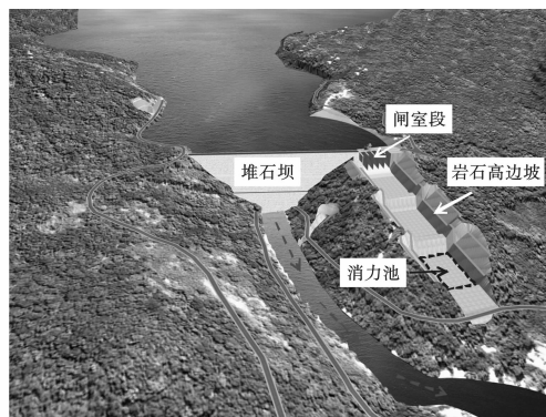
图1 南公1水电站首部枢纽及溢洪道布置图 Fig. 1 Layout of head hydroproject and spillway of Namkong 1 Hydropower Station
