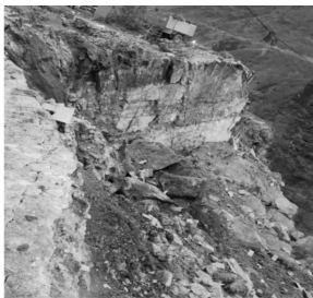
(a) 相对完整岩体的爆后效果 (a) Effect of relatively intact rock mass after blasting
