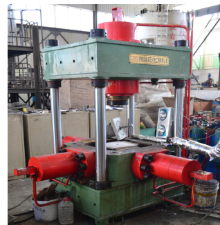
(c)真三轴围压加载系统
