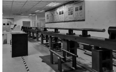
图1 中国矿业大学(北京) SHPB 实验系统 Fig. 1 SHPB experimental equipment in China University of Mining and Technology, Beijing
