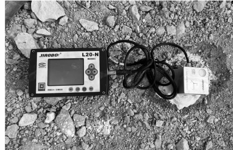
(b) 距爆心 4 m 处监测点 (b) Monitoring point at 4 m from the center of the explosion
