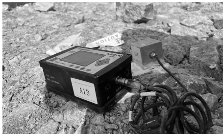
(c) 距爆心 6 m 处监测点 (c) Monitoring point at 6 m from the center of the explosion
