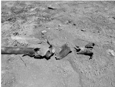
图5 30 cm 间隔连续传爆效果 Fig. 5 Continuous detonation effect with 30 cm decking
