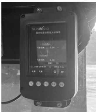
图 3 凿岩航道钻智能显示系统 Fig. 3 Intelligent display system for chiseled channel drilling
