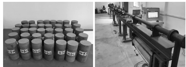
(a) 标准试件 (a) Standard specimen (b) SHPB 压杆装置 (b) SHPB lever device
