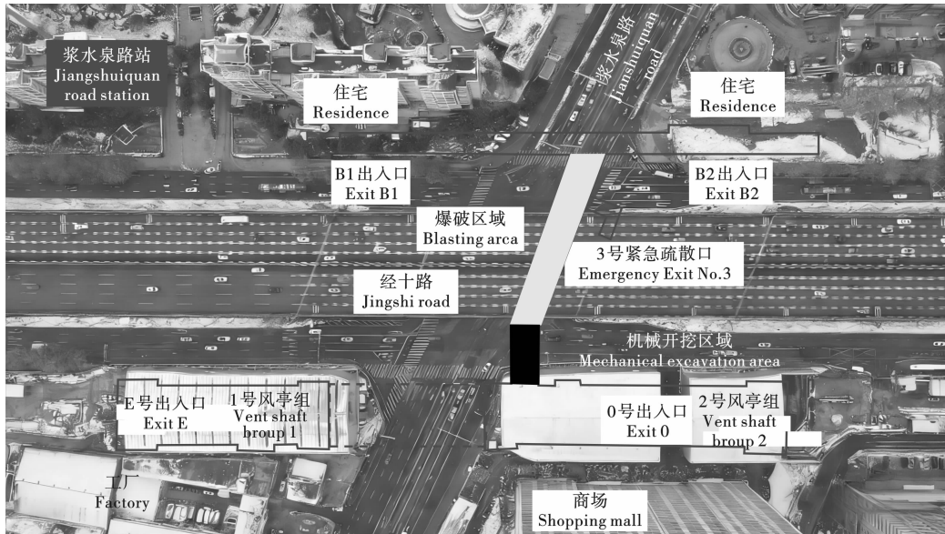
图1 浆水泉路站总平面布置图 Fig. 1 General layout of Jiangshuiquan Road Station
