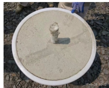
(c) 混凝土养护 28 d (c) Concrete curing 28 days
