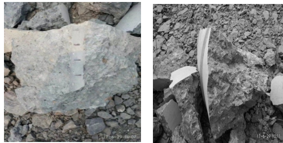
(a) 残留炮孔 (b) 极大块形状 (a) Hole shape (b) Block size
