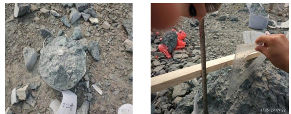
(a) 残留体形态 (b) 统计体积及节理裂隙 (a) Residual body (b) Counting volume and joints
