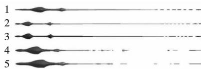
图8 无壳体和壳体壁厚线性变化的聚能射流形态图 Fig. 8 Morphological diagram of shaped charge jet without shell (No. 1) and with varying linearly wall thickness shell (No. 2~5)
