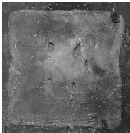
图 15 反应装甲爆炸的靶板塑性变形 Fig. 15 The plastic deformation of target plate under ERA explosion
