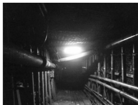
图 17 采用等长装药结构巷道留设效果 Fig. 17 Isometric charge structure and goaf retaining roadway
