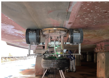
图 12 爬壁机器人上搭载的旋转除锈喷头试验快照 Fig.12 Experimental test snapshot of the rotary de-rusting sprayer device using a wall-climbing carrier platform
