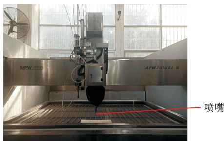
图 1 APW2016BA-18 五轴数控超高压水切割机 Fig.1 APW2016BA-18 five-axis CNC ultra-high pressure waterjet cutting machine
