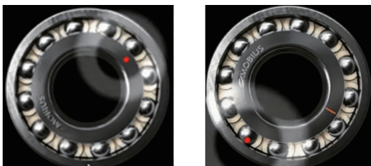
(a) 内圈故障 (b) 滚子故障
