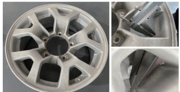
图 33 某企业机器人打磨后轮毂窗口边缘倒角尺寸测量 Fig.33 Dimensional measurements of chamfered wheel window edges after robotic grinding in enterprise
