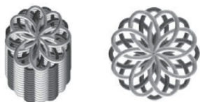
图 5 圆形截面编织结构 ( A = B ) Fig. 5 Braided structures with circular section ( A = B )
