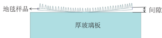
图 2 簇绒地毯翘曲测试示意 Fig. 2 Warping test indication of tufted carpet
