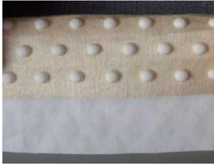
图5 硅胶点/芳纶水刺毡/PTFE 复合材料 Fig. 5 Silicone spots/Aramid felt/PTFE composite material
