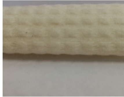
图6 芳纶凸起水刺毡/PTFE 复合材料 Fig. 6 Aramid raised felt/PTFE composite
