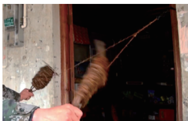
图 12 合绳工序实拍 Fig. 12 Photograph of the palm rope plying process
