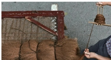
图 11 捻棕线工序实拍 Fig. 11 Photograph of the palm yarn twisting process
