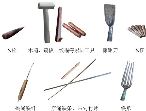
图 21 拉底绳、穿棕绳时采用的传统工具实物照片 Fig. 21 Photographs of the traditional tools used in palm rope weaving
