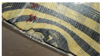
图5 织物滑移 Fig. 5 Fabric slippage
