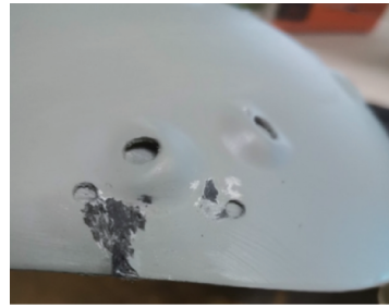
图 9 局部纤维出现挤伤 Fig. 9 Local fibers exhibited crushing injury
