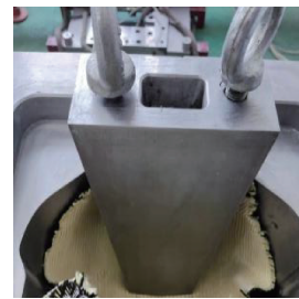
图6 压前部铺后部 Fig. 6 Press the front part and lay-up the rear part
