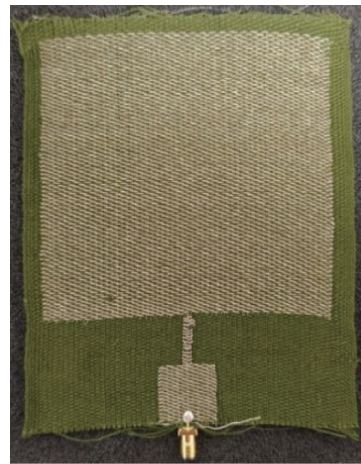
图 3 织物微带贴片天线试样 Fig. 3 Sample of the fabric microstrip patch antenna
