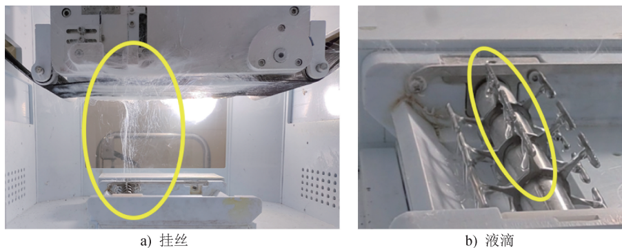
图 3 质量分数 26% 的 PVA 纺丝液无针纺过程中的纤维状态和纺丝液状态 Fig. 3 Fiber state and spinning solution state during NLE of PVA spinning solution with a mass fraction of 26%
