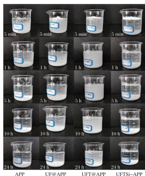
图5 改性前后APP的水溶性测试光学照片 Fig.5 Optical photos of water solubility test of APP before and after modification
