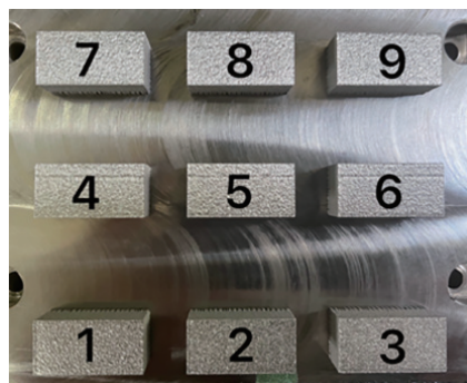
图1 SLM成形的TC4-x316L试样
