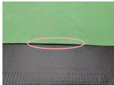
图 13 0.095 MPa 压实后蜂窝边缘配合状态 Fig. 13 0.095 MPa compacted honeycomb edge coordination state
