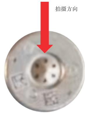
图 5 喷油器喷孔布置与拍摄方向 Fig.6 Injector nozzle layout and shooting direction
