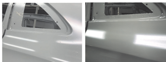
a. 枪嘴更换前PVC残胶飞溅 b. 枪嘴更换后无PVC残胶
