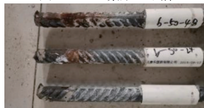
(c) RC-6-50-锈蚀 48 h 试件
