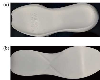
图 12 (a) P4HB-PUF 鞋中底正面和 (b) P4HB-PUF 鞋中底背面 Fig. 12 (a) Front and (b) back views of the P4HB-PUF shoe midsole
