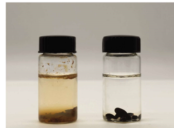
图6 KL/PVA-S100及KLS2/PVA-S100在凝固浴中的照片 Fig.6 Photograph of KL/PVA-S100 and KLS2/PVA-S100 in a solidification bath
