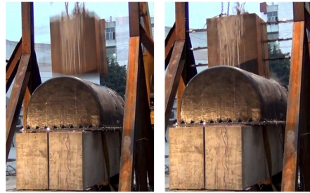
Fig. 12 Deformation at the impact point of the fender
