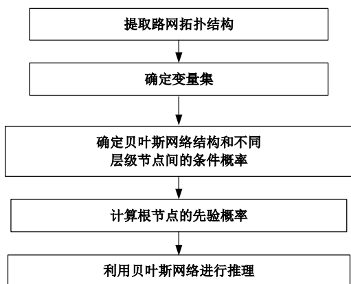
图 1 基于贝叶斯网络的道路交通网络模型构建方法 Fig. 1 A method for constructing a road traffic network model based on Bayesian networks
