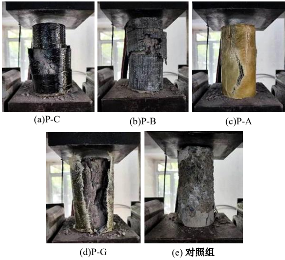
图 11 FRPs 加固试件及对照组试件抗压破坏状态 Fig. 11 Compressive failure state of FRP reinforced specimens and control group specimens
