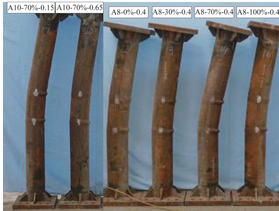
图7 代表性试件的整体破坏模式 Fig. 7 Overall failure modes of representative specimens
