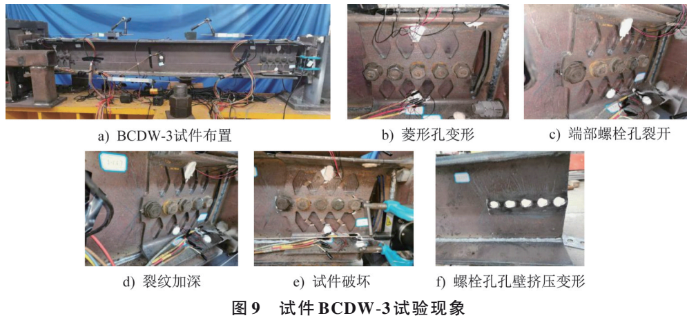
Fig. 9 Test phenomenon of specimen BCDW-3
